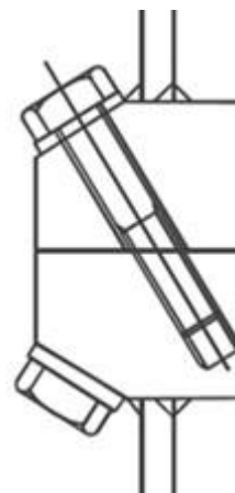
Figure 8 Bolted X-joint. (Source: Alexander Jakubowski, 2003 dissertation).
