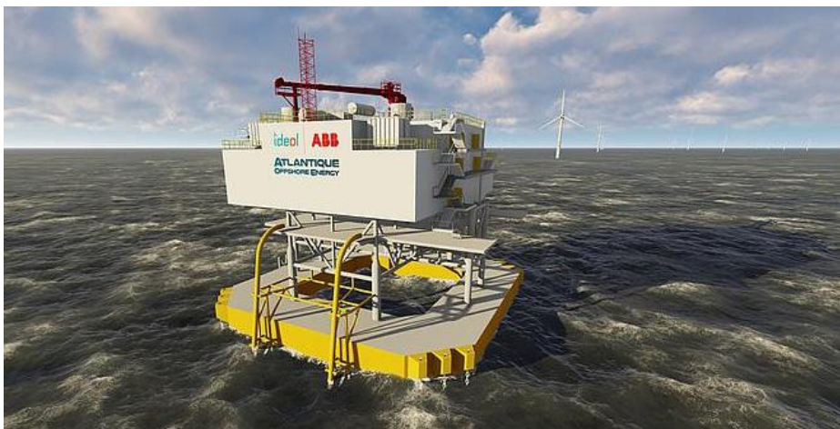
Figure 36 Floating offshore substation: potential solution announced by Ideol in 2019. (Source: Windpower Monthly).
