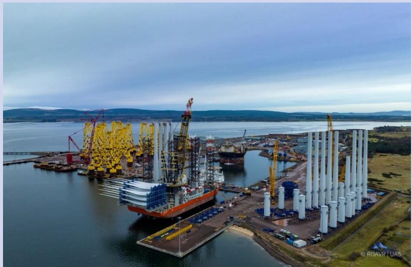
Jackets and towers staged at the Port of Nigg. Image courtesy of ROAVR group.
