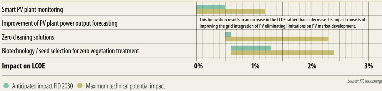
Table 8.2 Anticipated and potential impact of OMS innovations for a ground mounted utility scale PV plant using High Efficiency c-Si technology with FID in 2030, compared with an installation with the same nominal power on the same Site Type with FID in 2015.
