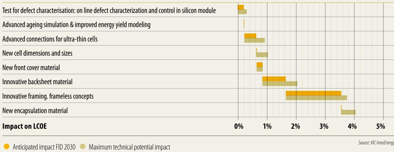
Table 5.2 Anticipated and potential impact of PV module manufacturing innovations for a rooftop PV installation using High Efficiency c-Si technology with FID in 2030, compared with an installation with the same nominal power on the same Site Type with FID in 2015.
