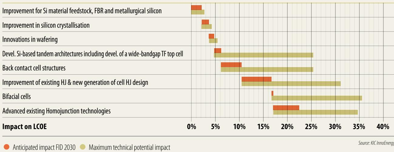
Table 4.2 Anticipated and potential impact of PV cell manufacturing innovations for a rooftop PV installation using High Efficiency c-Si technology with FID in 2030, compared with an installation with the same nominal power on the same Site Type with FID in 2015.
