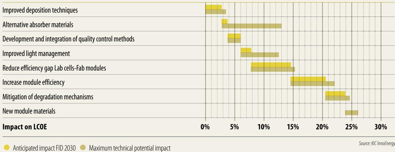
Table 6.1 **Anticipated and potential impact of TF module innovations for a ground mounted PV installation using TF technology with FID in 2030, compared with an installation with the same nominal power on the same Site Type with FID in 2015.**
