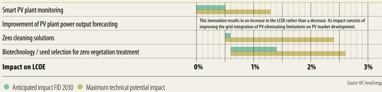
Table 8.1 Anticipated and potential impact of OMS innovations for a ground mounted utility scale PV plant using conv c-Si technology with FID in 2030, compared with an installation with the same nominal power on the same Site Type with FID in 2015.
