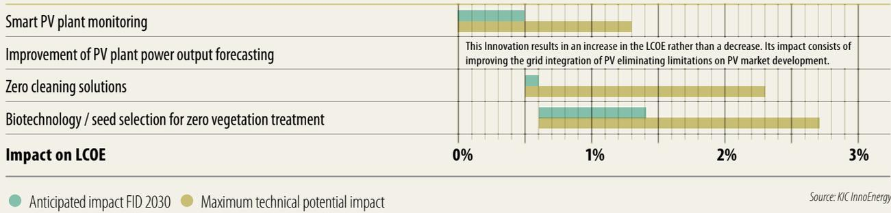
Table 8.3 Anticipated and potential impact of OMS innovations for a ground mounted utility scale PV plant using TF technology with FID in 2030, compared with an installation with the same nominal power on the same Site Type with FID in 2015.
