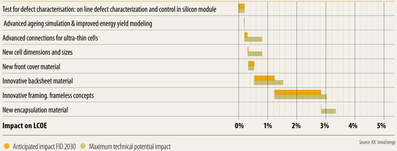
Table 5.1 Anticipated and potential impact of PV module manufacturing innovations for a ground mounted utility scale PV plant using Conventional c-Si technology with FID in 2030, compared with an installation with the same nominal power on the same Site Type with FID in 2015.
