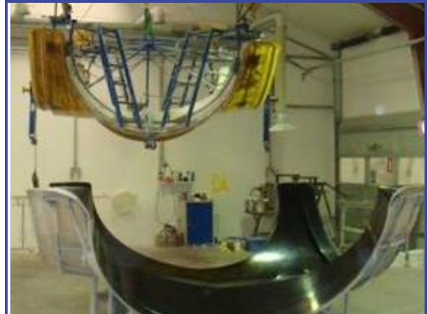
Figure 5.2.1 Resin transfer mould tooling for a spinner.
