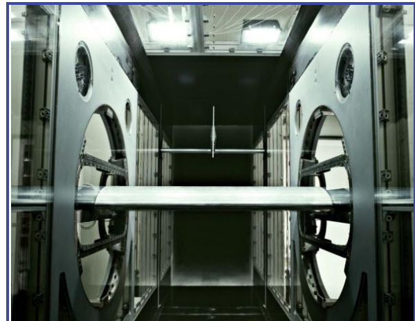
Figure 4.2.6 Wind tunnel testing on a wind turbine blade section.
