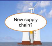
Float-out-and-sink Avoid offshore crane cost
