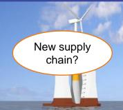
**Float-out-and-sink** Avoid offshore crane cost
