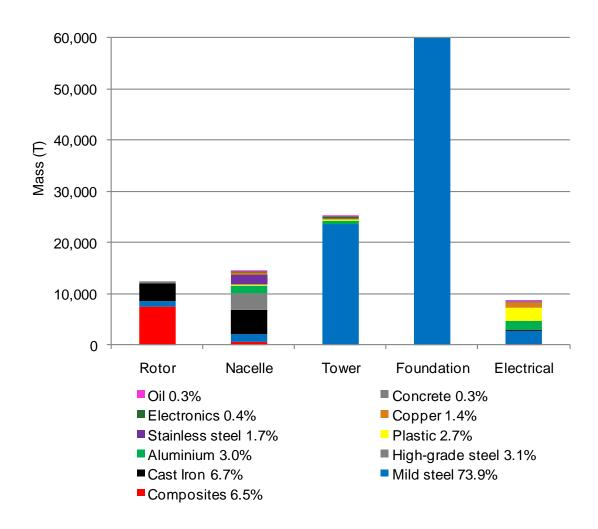
Material breakdown for a 500MW wind farm.
