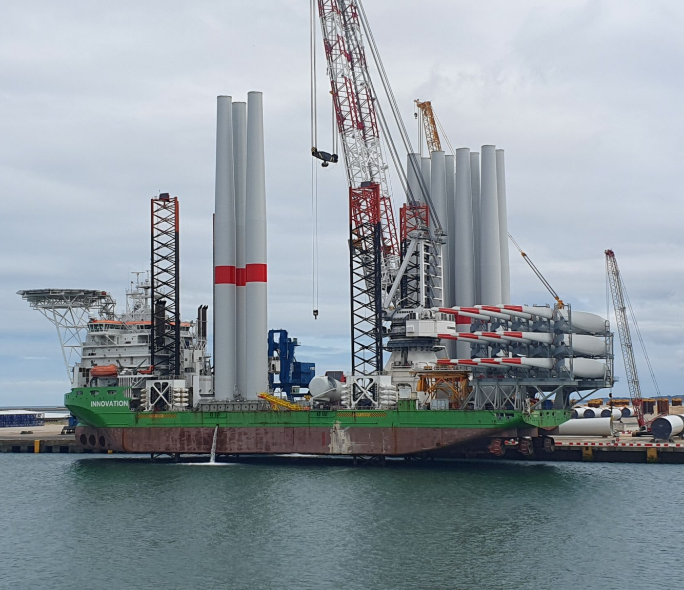
Deme Innovation loading turbines for installation
